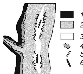
Fig. 4. Morphology of quartz veins: 1 – sulphides; 2 – fine-grained, cryptocrystalline quartz; 3 – coarse-crystalline quartz; 4 – fluorite; 5 – barite; 6 – vug.
