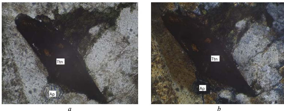
Fig. 10. Titanite (Ttn) and apatite (Ap) in Osnytskiy granite, field of view – 2 mm: a – PPL; b – XPL.
