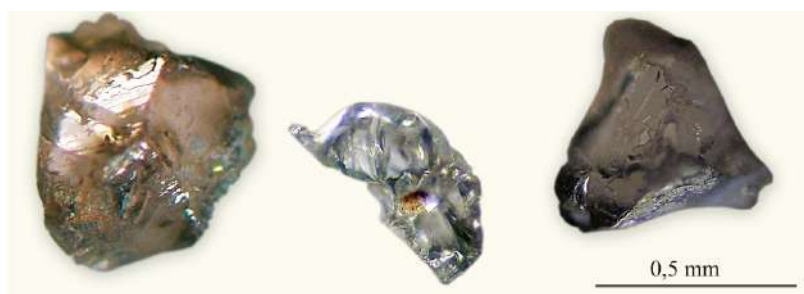
Fig. 5. Micrographs of Ti 3+ -bearing corundum
